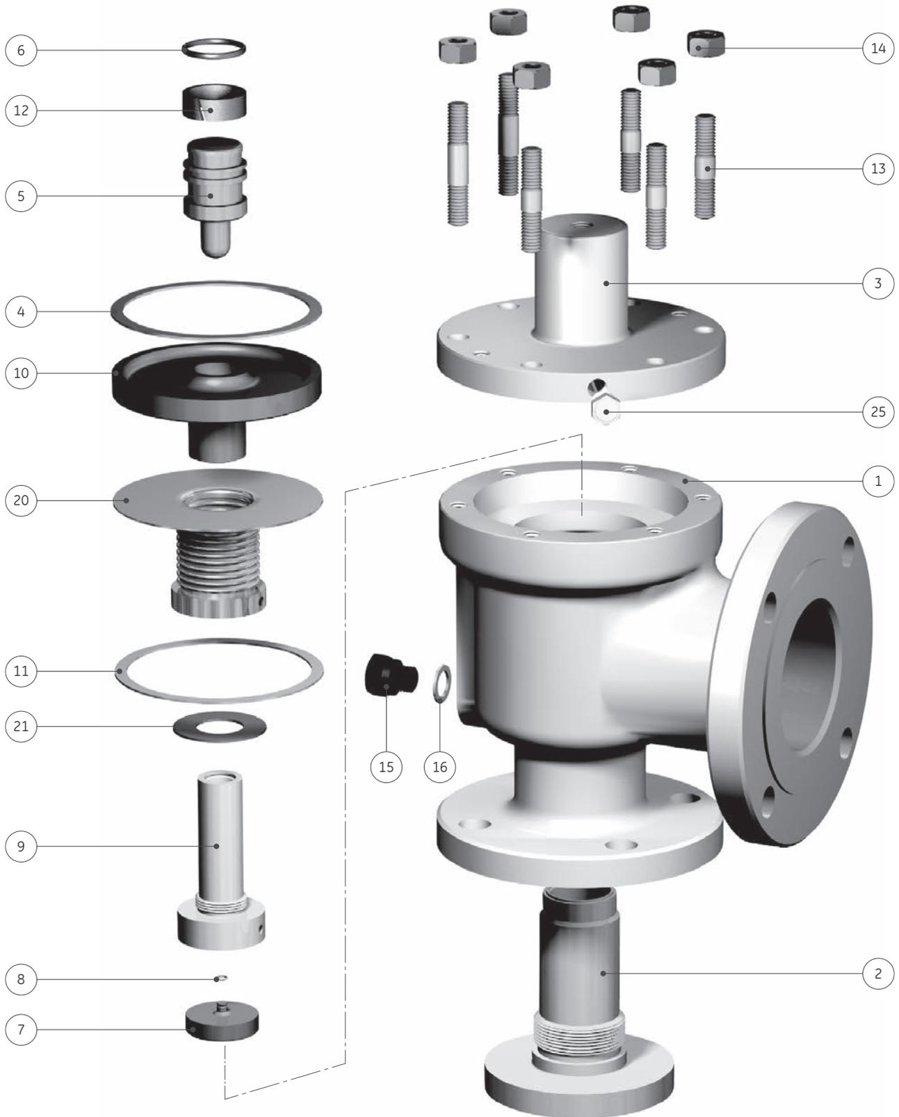
Figure 23: Bellows Metal Seat Valve Disassembly
