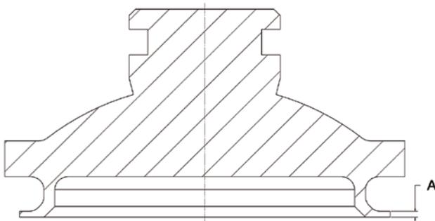
**Figure 45: UM Cryogenic Disc Design (D-U Orifices)**
