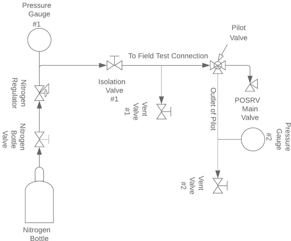
**Figure 73: Typical Installation Arrangement with Auxiliary Supply for Artificial Actuation of Pilot Only**
