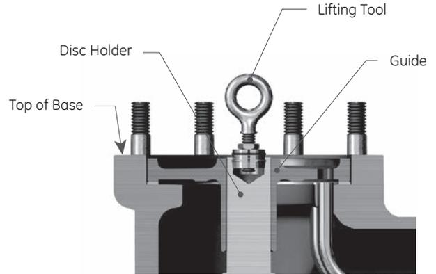
**Figure 27: Disc Holder Removal Tool (P-U)**
