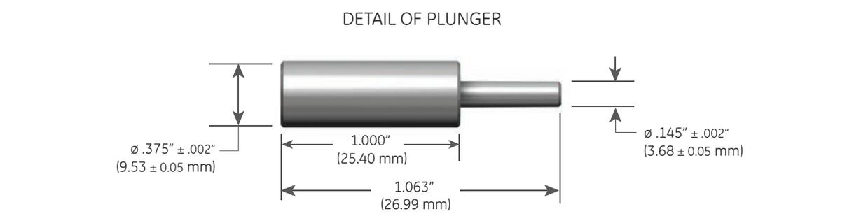
**Figure 92: Adjuster Top Seal Insertion Tool**
