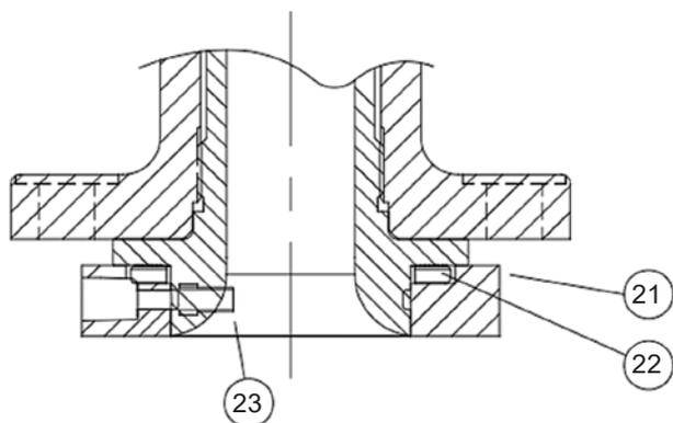
**Figure 7: Main Valve Construction - Integral Sense**
