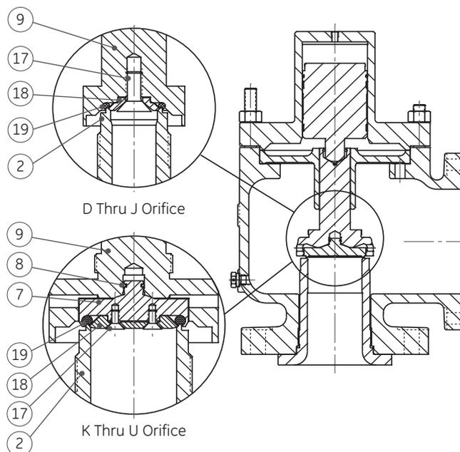
Figure 2: Main Valve Construction - Soft Seat
