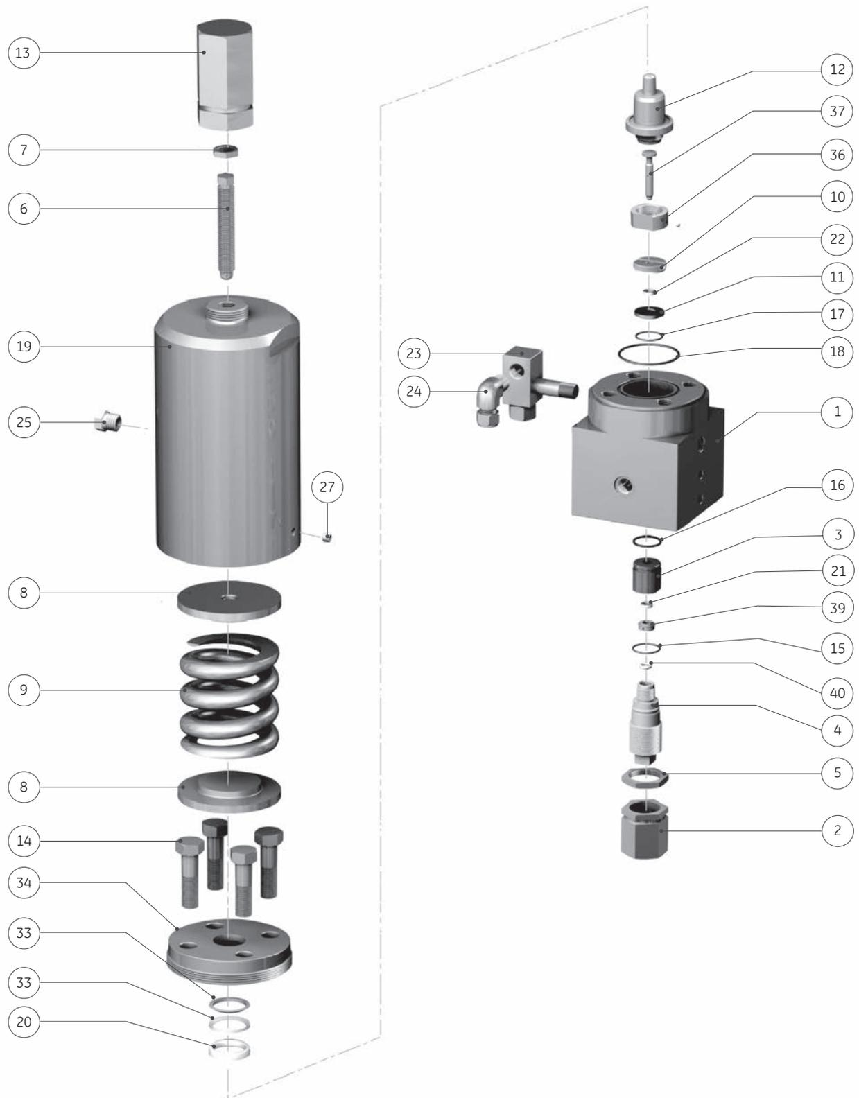
Figure 55: 39MV72 Disassembly
