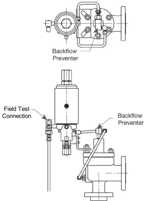
Figure 74: Field Test Connection / Backflow Preventer Option
