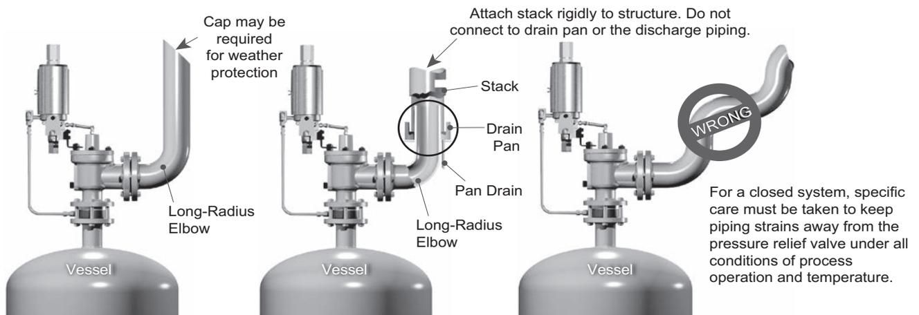
**Figure 19: POSRV Parts Alignment**
