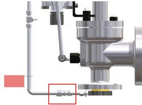
**Figure 17: Integral Sensing Tubing Union and Tag**
