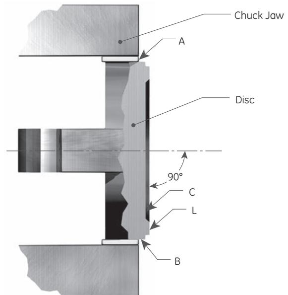
Figure 40: Standard Disc Seating Surface
