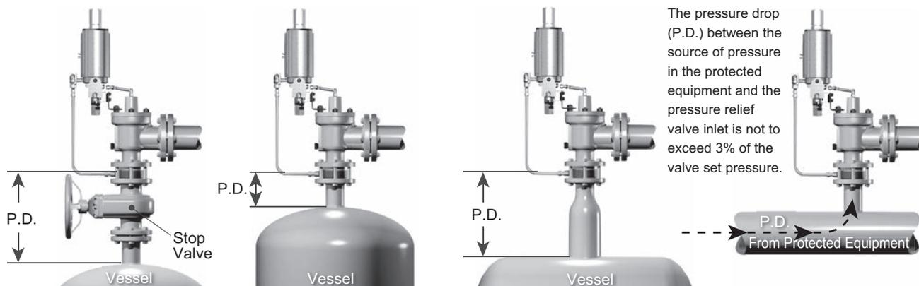
Figure 16: Pressure Drop on the Inlet Piping
