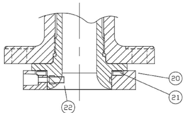
Figure 3: Main Valve Construction - Integral Sense
