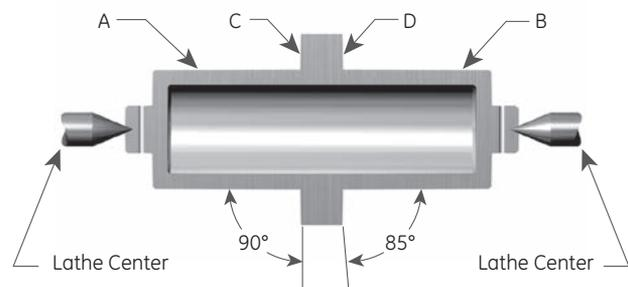
Figure 38: Nozzle Lap in a Lathe
