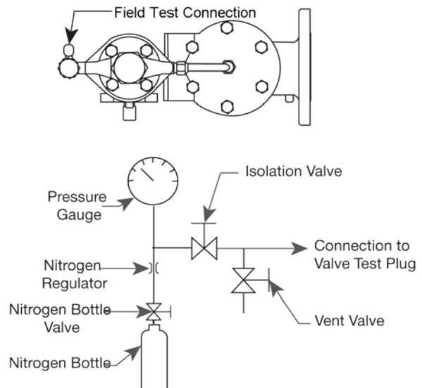
Figure 69: Typical Field Test Arrangement
