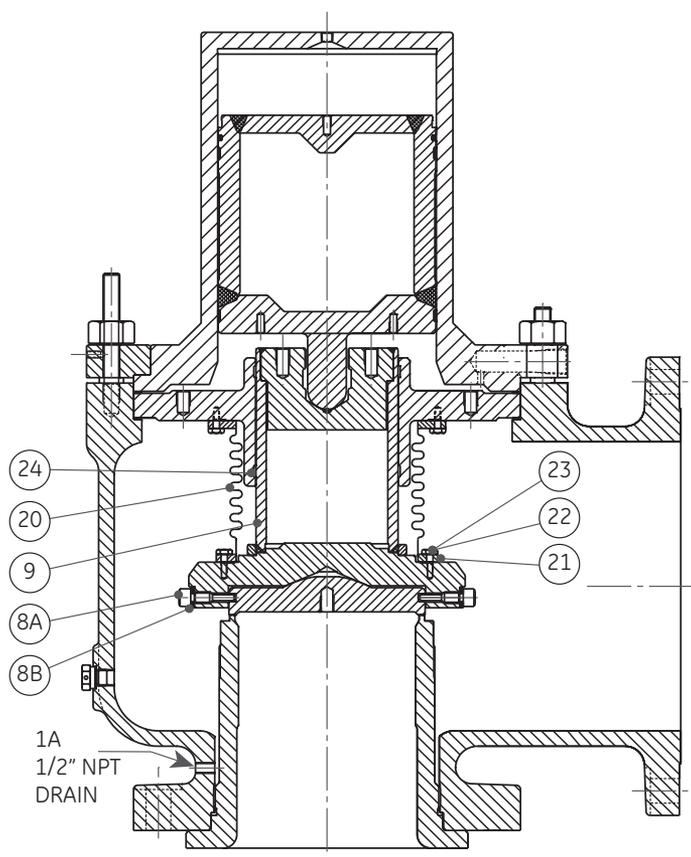
Figure 5: Main Valve Construction - Bellows (V&W orifices)
