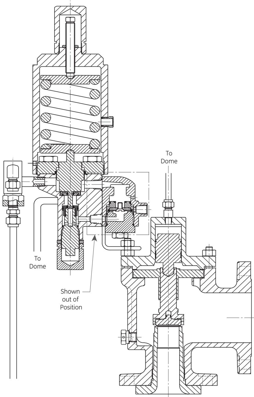
Figure 14: MV07 Valve Closed (Normal Position)
