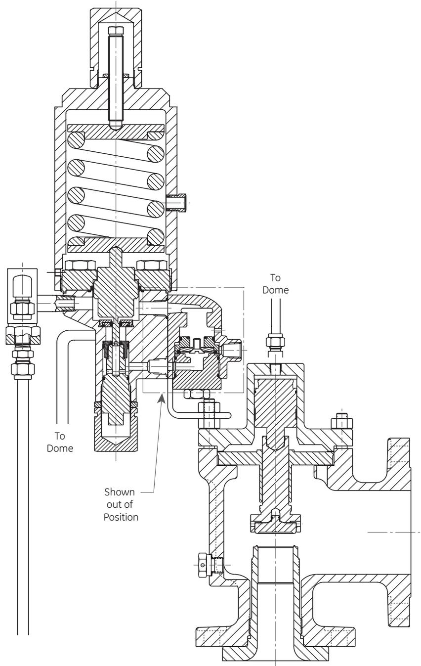
Figure 15: MV07 Valve Modulating (Partial Relieving Position)
